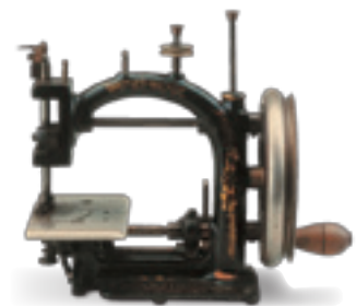
Chain-Stitch Sewing Machine for the Production of Straw Hats
