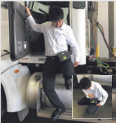
▲ An employee conducting a wearability test of the prototype when getting on and off a customer's delivery truck
