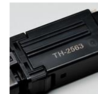
Printing lot numbers on switch parts
