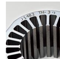
Printing production information on motor parts
