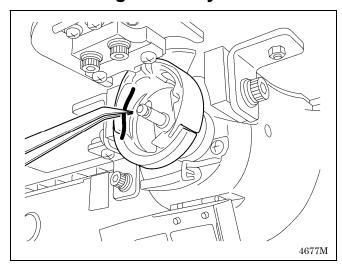
Remove the bobbin case, and then remove the thread scraps and lint from around the shuttle.
