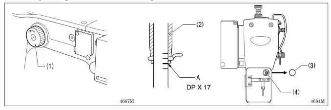
Turn the pulley (1) by hand in the direction of the arrow to move the needle bar to the lowest position. Then remove the rubber plug (3), loosen the screw (4) and then move the needle bar up or down to adjust so that the second reference line from the bottom of the needle bar (reference line A) is aligned with the lower edge of the needle bar bush (2).
