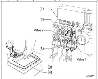
You can adjust the lifting and lowering speeds for the work clamps using the knobs (1) and (2) on valves 1 and 2.
