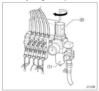
Lift up the handle (2) of the regulator (1) and then turn it to adjust the air pressure to  $0.5\,\mathrm{MPa}$ .
