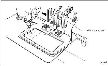
Move the work clamp arm all the way to the right when looking from the front of the sewing machine (the direction of the arrow in the illustration), and then gently tilt back the machine head.
