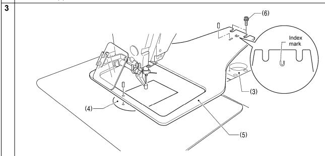
Use a 2 mm diameter pin to align the holes in the X feed bracket (3) and the needle plate (4) with the two holes in the feed plate (5), and then tighten the two bolts (6).
