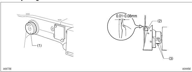
Turn the pulley (1) in the direction of the arrow to align the rotary hook tip (2) with the center of the needle, and then loosen the two set screws (3) and move the rotary hook forward or back to adjust so that the clearance between the needle and the rotary hook tip (2) is 0.01 to 0.08 mm.
