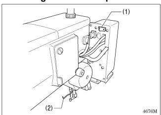
The thread wiper switch (1) can be used to turn the thread wiper (2) on and off.
