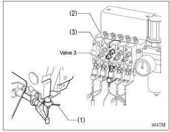
Valve 3 is used for adjusting the operating speed of the thread wiper (1).
