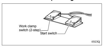
When the work clamp switch (left side) is depressed, the work clamp will be lowered, and when the start switch (right side) is depressed, the sewing machine will start.
