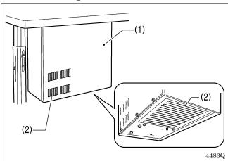
Use a vacuum cleaner to clean the filter in the air inlet ports (2) of the control box (1) at least once a month.
