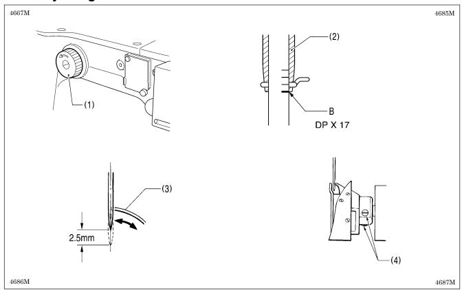
Turn the pulley (1) by hand in the direction of the arrow to raise the needle bar from the lowest position until the lowest reference line on the needle bar (reference line B) is aligned with the lower edge of the needle bar bush (2), and then loosen the two set screws (4) and move the rotary hook to adjust so that the rotary hook tip (3) is aligned with the center of the needle.
