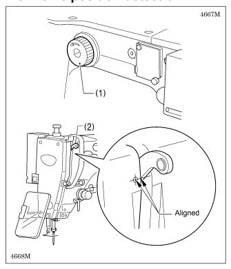
Before starting home position detection, check that the needle bar is at its highest position.
