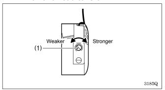
Adjust the lower thread tension by turning the adjusting screw (1).
