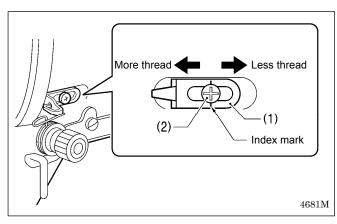
The standard position of arm thread guide R (1) is when the screw (2) is aligned with the index mark.
