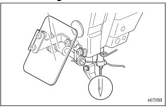
Always check that the tip of the needle is not broken and also that the needle is not bent before starting sewing.
