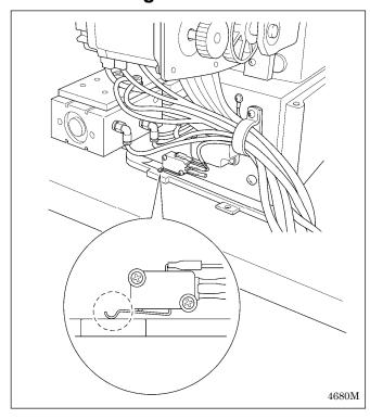
Check that the machine head switch is turned on as shown in the illustration.
