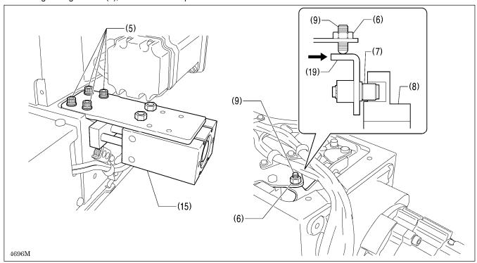
6. Loosen the four bolts (5) and the nut (6) until the thread trimmer roller (7) is within the groove in the thread trimmer cam (8). After this, tighten the set screw (9) until the thread trimmer roller (7) is touching the inside of the groove in the thread trimmer cam (8) and then turn it back in the counterclockwise direction by approximately 1/4 of a turn. Then tighten the nut (6).
