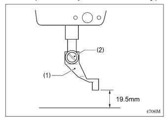
Install the intermittent presser foot (1) with the screw (2) so that the distance from the bottom of the intermittent presser foot to the top of the needle plate is 19.5 mm when the sewing machine is stopped and the intermittent presser foot (1) is raised.
