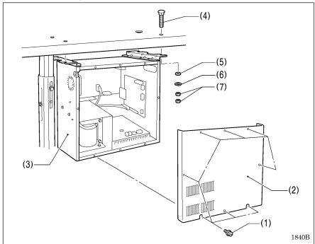
Remove the eight screws (1), and then remove the control box cover (2).
