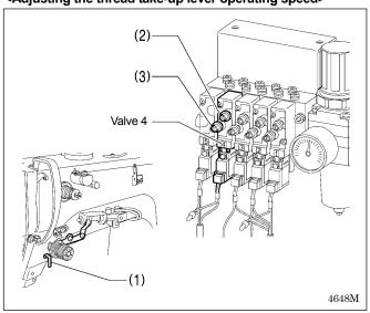
Valve 4 is used for adjusting the operating speed of the thread take-up lever (1).
