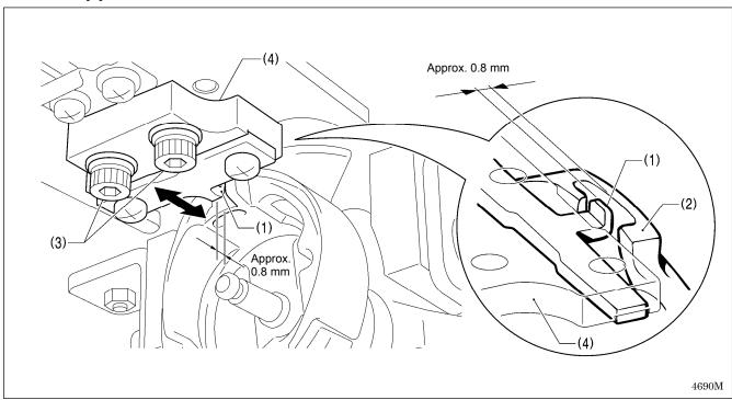
Loosen the two screws (3) and move the hook stopper setting base (4) to adjust so that the tip of the hook stopper (1) is approximately 0.8 mm away from the needle drop surface of the inner hook (2).
