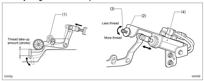
At the time of shipment from the factory, the thread take-up amount (stroke) of the thread take-up lever (1) is adjusted to the standard amount of 5 mm. Adjust this amount according to the sewing conditions to prevent the thread from pulling out at the sewing start.
