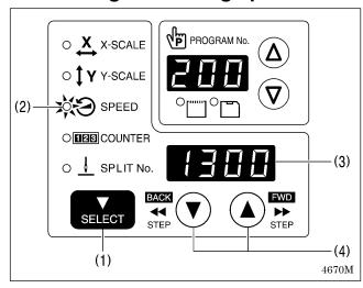
The sewing speed is set to 1300 (sti/min) at the time of shipment from the factory.
