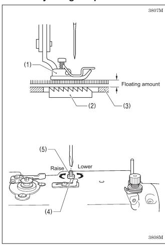
When sewing stretch materials and materials with long pile, you can make minute adjustments to the floating amount for the presser foot (1) in accordance with the material.
