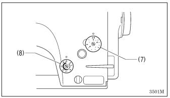
5. Turn the stitch length dial (7) and the condense dial (8) to the maximum feed amount for the feed dog being used. (Set the condense dial (8) to a negative number.)
