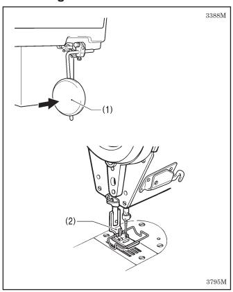
The presser foot (2) can be raised by pressing the knee lifter plate (1).
