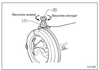
The presser foot pressure should be as weak as possible, but strong enough so that the material does not slip.
