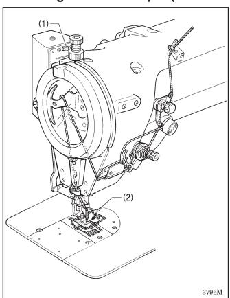
Press the thread wiper switch (1) to the • side. If this is done, the thread wiper (2) will operate after the thread is trimmed.
