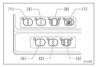
Press the sewing pattern select keys ([1] to [7] in the illustration left) to select the sewing pattern. The indicator for the key that was pressed will illuminate and the pattern number that has been set for that key will appear in the main display.
