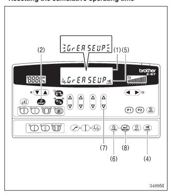
After the grease has been applied, carry out the following procedure to reset the cumulative time between grease applications.
