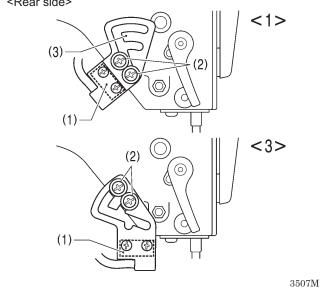
The installation position of the actuator (1) can be adjusted as shown in the illustration.
