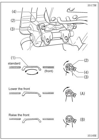
The standard angle for the feed dog (1) is for the top of the needle plate to be parallel with the top of the feed dog (1) (for the 8550A) or raised slightly at the side closest to the operator (for the 8560A) when the feed dog (1) is raised to its highest position above the needle plate. (with the O mark on the feed bracket shaft (2) aligned with the mark on the feed rocker bracket arm (3)).
