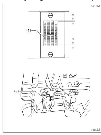
The clearance between the feed dog (1) and the needle plate should be the same at the front and back of the feed dog (1) when the feed dog (1) is moved to its furthest forward and furthest back positions by turning the machine pulley.
