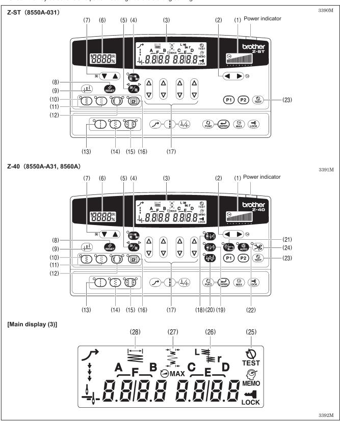
The power indicator illuminates when the power switch is turned on.
