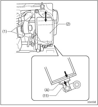
9. For models/specifications other than the 8550A-031, with the reverse lever (9) lowered all the way (with the plunger (11) of the quick reverse solenoid moved to its highest position), touch the quick reverse solenoid (2) against section (A) of the plunger (11), and then tighten the two screws (1).
