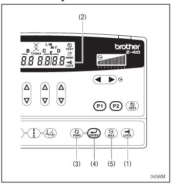
When the power switch is turned on, the LOCK key (1) turns ON. (The icon (2) is illuminated.)
