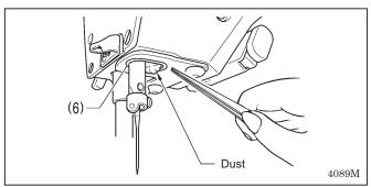
10. If any dust has collected near the stopper (6), use tweezers or a similar tool to remove it.
