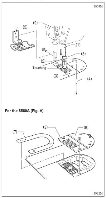
With the accessory needle bar height gauge (2) installed to the needle bar (1), adjust so that the needle bar height gauge (2) is touching the top of the needle plate (3) when the needle bar is at its lowest position.
