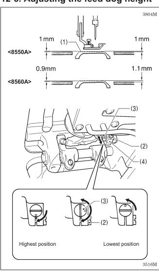
The standard height of the feed dog (1) when it is raised as far as possible above the surface of the needle plate is as given below.
