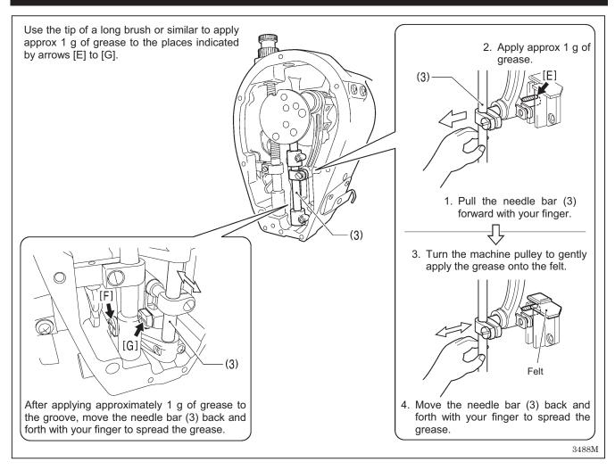
After applying grease in the places indicated by arrows [A]-[G] above, carry out the reset operation described below.
