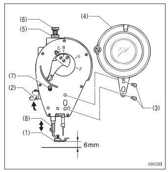
The standard height of the presser foot (1) is 6 mm when the presser foot (1) is raised by means of the presser bar lifter (2).
