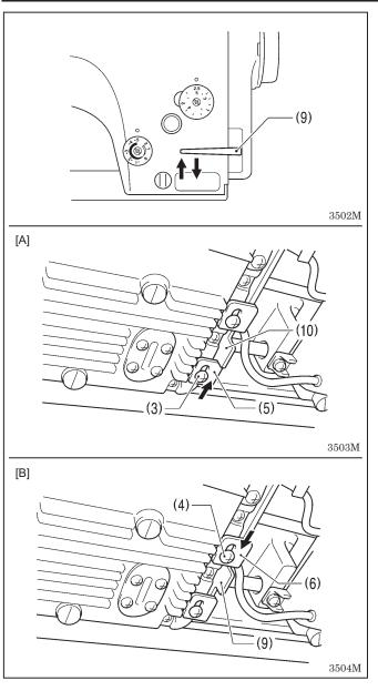
Check that the feed dog does not touch the needle plate both when the reverse lever (9) is not lowered and when it is lowered.
