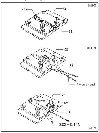
Adjust the tension of the lower thread presser spring (1) so that the tension is 0.03 to 0.11 N when the lower thread presser spring (1) is pulling the lower thread (nylon thread: 100D 1 X 3 (Z)) after thread trimming.
