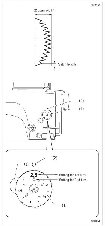
Turn the stitch length dial (1) until the desired stitch length number is aligned with the index mark (2) above the dial.
