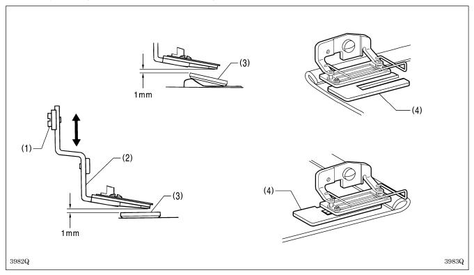
Loosen the screw (1), and then move the upper thread trimmer (2) up or down to adjust the clearance between the upper thread trimmer (2) and the work clamp (3) to approximately 1 mm.
