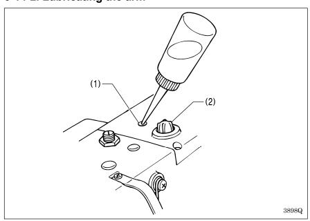
Apply 5-6 drops of oil to the oil inlet (1) at the top of the arm.
