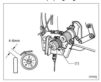
Loosen the set screw (1), and turn the entire thread tension adjuster to adjust the thread take-up spring height to between 4 - 6 mm in accordance with the material to be sewn.
