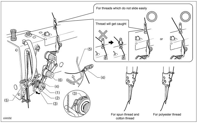
Thread the upper thread correctly as shown in the illustration.
