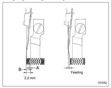
Because the needle and cutter positions are separated by 2.2 mm as shown in the illustration, the distance between the edge of the front tack and the edge of the buttonhole cannot be set to less than 2.2 mm.
