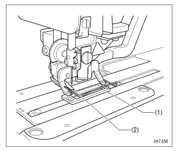
2. Remove lint and dust from around the work clamp (1) and upper thread trimmer (2).
