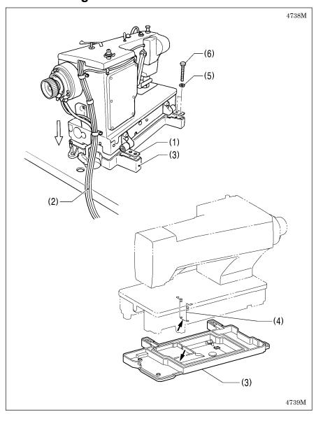
Place the two bed hinges (1) so that they are level as shown in the illustration at left, and then place the machine head gently on top of the bed base (3) so that the cables (2) do not get clamped.
