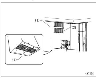
Use a vacuum cleaner to clean the filter in the air inlet port (2) of the control box (1) at least once a month.
