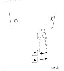
If you press the lacktriangledown key while in threading mode, the needle will return to the middle position.
