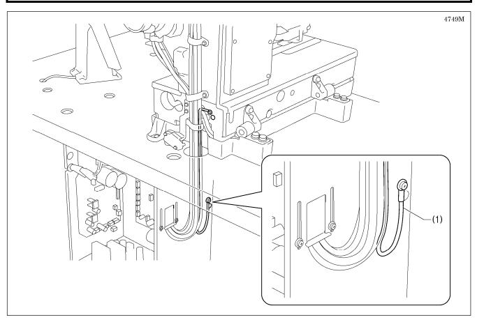
(1) Ground wire from the machine head (Ground mark position)
