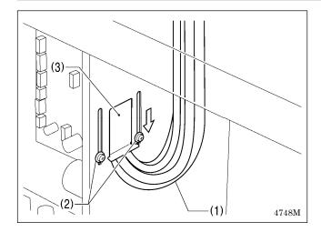
4. Close the cord presser plate (3) in the direction of the left arrow, and secure it by tightening the two screws (2).
