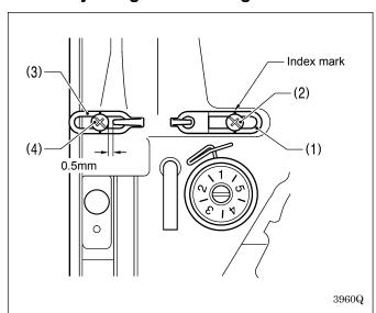
The standard position of arm thread guide (1) is when the screw (2) is aligned with the index mark.
