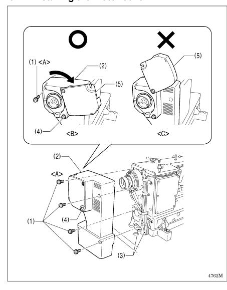
1. Install the motor cover (2) with the three screws (1) (other than <A>).
