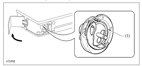
When first installing the machine and when the machine has not been used for an extended period of time, remove the bobbin and add 2-3 drops of oil to the rotary hook race (1) before sewing.
