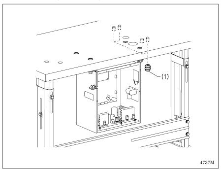
Install the four flange nuts (1) to the underside of the work table.
