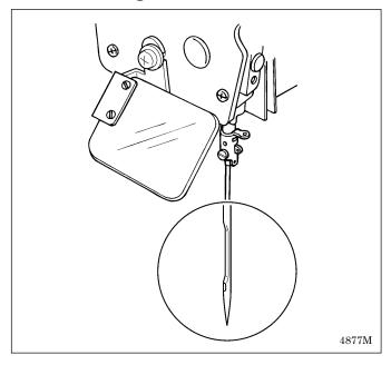
Always check that the tip of the needle is not broken and also the needle is not bent before starting sewing.
