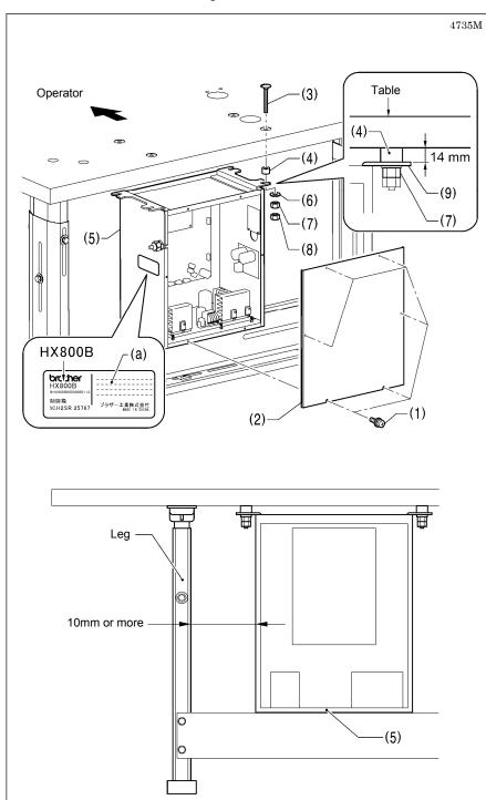
Remove the six screws (1), and then remove the control box cover (2).
