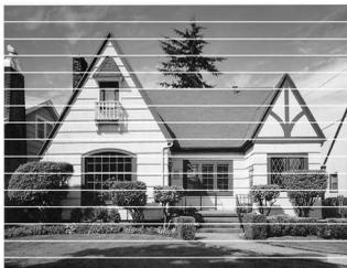
When an print head nozzle is clogged the printed sample looks like this.
