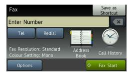
3 You can change the following fax-sending settings. Press Options. Swipe up or down, or press ▲ or ▼ to scroll through the fax settings. When the setting you want is displayed, press it and choose your new option. When you are finished changing the options, press OK.
