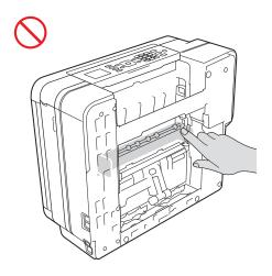
Do not apply pressure with your hand or elbow in the gray shaded area shown in the illustration below. Doing so may cause the ADF document support (1) to inadvertently open.
