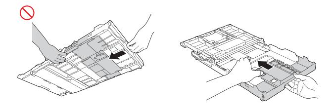
DO NOT touch the edges of the metal parts behind the rollers in the gray shaded area shown in the illustration. These parts have sharp edges and doing this may cause injury to your fingers by cutting them.
