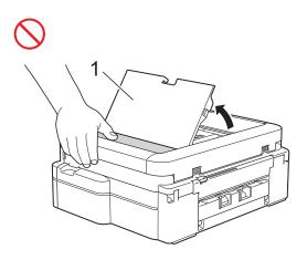
DO NOT carry the product by holding the scanner cover, the Jam Clear Cover, the manual feed slot cover, or the control panel. Doing this may cause the product to slip out of your hands and may result in injury.
