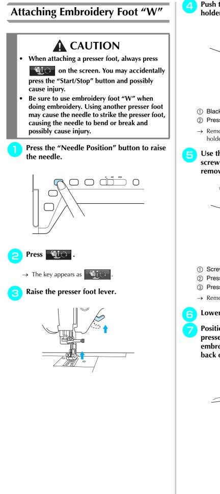
Push the black button on the presser foot holder and remove the presser foot.
