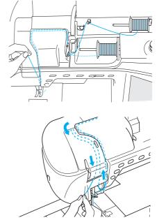
Do not pass the thread in the needle bar 8 thread guides on the needle bar. Thread the needle on the right side.
