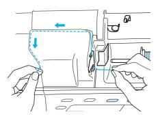
When finished pulling the thread through the thread guide, cut the thread and leave the thread in position.
