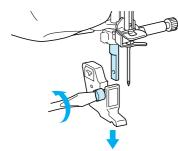
Set the operation lever of the walking foot so that the needle clamp screw is set between the fork, and position the walking foot on the presser foot bar.
