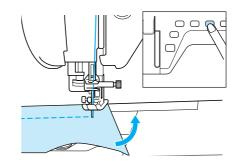
When edge stitching a short stitch length close to the edge of the fabric, the presser foot may not cover enough fabric for proper feeding. Before you begin to sew, sew a basting thread at the corner point. When you change direction at the corner, start sewing as you pull the basting thread toward the back.
