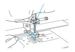
Pull up the bobbin thread, then pass it 5 under the presser foot and pull it about 100 mm (approx. 3-4 inches) toward the back of the machine, making it even with the upper thread.
