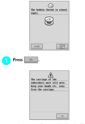
→ The carriage will move and the thread will be automatically cut.
