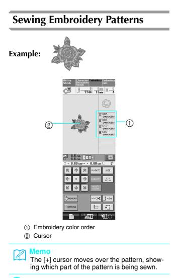
Thread the machine with the first color (see "Threading Using the "Automatic Threading" Button" on page 25).
