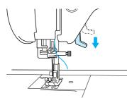
Holding the thread with both hands, pass the thread through both the upper and lower needle bar thread guides.
