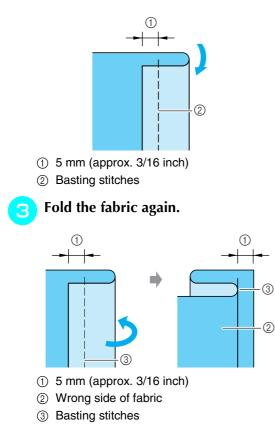
Attach blind hem stitch foot "R", and lower the presser foot. Position the fabric so the folded edge touches the guide of the presser foot.
