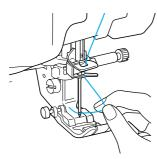
Pass the thread through the presser foot, and then pull out about 100-150 mm (approx. 4-6 inches) of thread toward the back of the machine.
