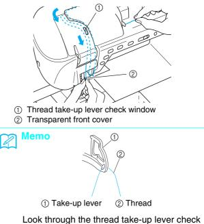
Look through the thread take-up lever check window and check that the thread is correctly fed through the take-up lever, turning the handwheel toward you.
