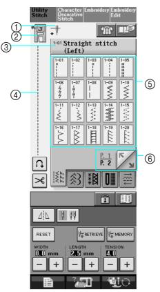
① Shows single or twin needle mode setting, and the needle stop position.
