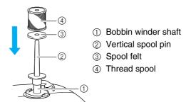
Install the spool felt and the thread spool in that order, and then thread the upper thread.
