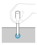
When using the eyelet punch, place thick paper or some other protective sheet under the fabric before punching the hole in the fabric.
