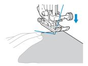
Press (†) (Start/stop button) or press down on the foot controller.
