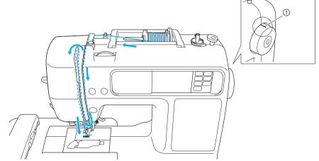
① Mark on handwheel
