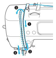
Make sure that the thread is passed into the thread take-up lever as shown below.
