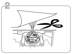
Cut the entangled thread with small scissors above the needle plate and then gently remove the thread and fabric.
