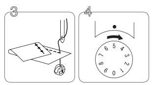
Upper tension is too loose. (Locks appear on the reverse side of the fabric.) Increase the tension by turning the dial a higher number.
