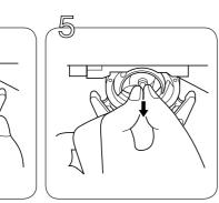
Remove the hook by grasping the center post and pulling out. Note it's position related to the driver.
