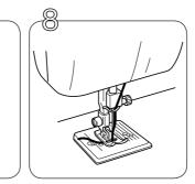
Thread the needle from front to back and pull out about 2" of thread.
