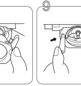
Remove the retaining ring.
