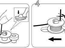
While holding the end of When the bobbin is full, it the thread, depress the will stop winding. Cut the thread, slide the winding shaft to the left and remove the bobbin.
