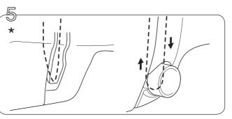
Pass the thread into the thread tension discs or \*behind the thread tension dial from the right to the left.
