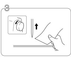
Turn the balance wheel to raise the needle, then remove the fabric.
