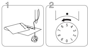
Upper thread tension is too tight. (Locks appear on the surface of the fabric.) Decrease the tension by turning the dial to a lower number.
