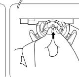
Grasp the center post of the hook, match the hook position opposite the driver and insert.
