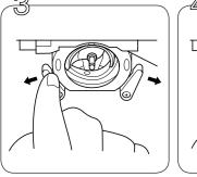
Slide the latch levers out from the retaining ring.
