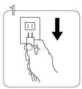
Remove the power plug from the outlet.
