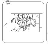
Raise the needle to its highest position and remove the bobbin case by pulling the latch.
