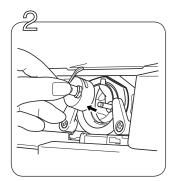
Raise the needle to its highest position, pull the latch and remove the bobbin case.
