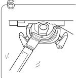
Remove any accumulated lint and thread with a brush.
