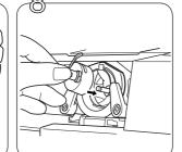
Holding the bobbin case by the latch align the finger with the top opening of the shuttle race , insert the case into the shuttle race and release the latch. The latch should hold the bobbin case in place.
