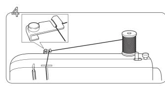
Pass the thread through the thread guide and down the right channel on the front of the machine.
