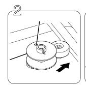
Pass the thread through the hole on the bobbin from inside, and slide the winding shaft to the right.
