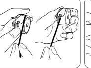
Pull the thread tail into the bobbin case groove, under the spring clip and into the thread guide hole.
