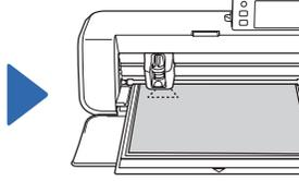
Press "Feed Button" to feed out the mat.
