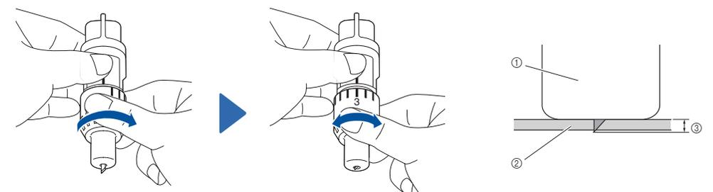
Fully turn the cap to the right to extend the blade tip to its maximum.
