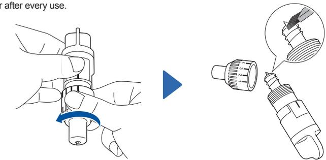
Twist off the holder cap to remove it.
