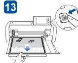
Press the "Feed" button in the operation panel to release the mat.
