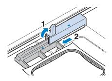
Insert a wound bobbin into the machine. (Refer to "Setting the Bobbin" on page 20.)
