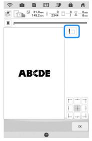
→ The needle is positioned in the lower-left corner of the pattern. The carriage moves so that the needle is positioned correctly.
