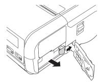
3 Close the battery cover, and then move the battery cover lock to the lock position.
