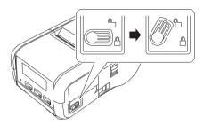
While pushing the battery latch, remove the battery.
