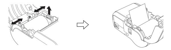
4 Close the media roll compartment by pressing down on the center of the cover until it locks into place.
