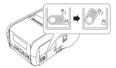
Insert the battery into the battery compartment until the battery latch locks into place. Make sure that the terminal end of the battery is facing inwards and oriented correctly as shown. Do NOT use excessive force to install the battery.
