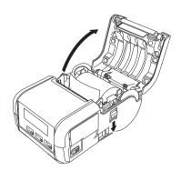
While pushing the roll release lever, tilt one of the roll guides slightly, and then remove the roll. The roll can be removed without changing the position of the roll guides.
