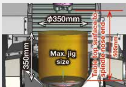
▲ Machining area larger than that of the previous model
