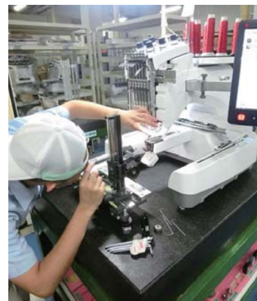
Adjustment with a microscope
