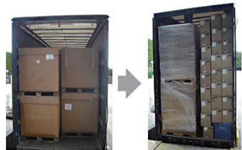
Improving the container loading rate (70% on the left, 95% on the right)
