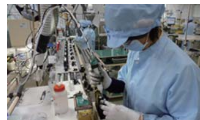
Process for reusing toner cartridges
