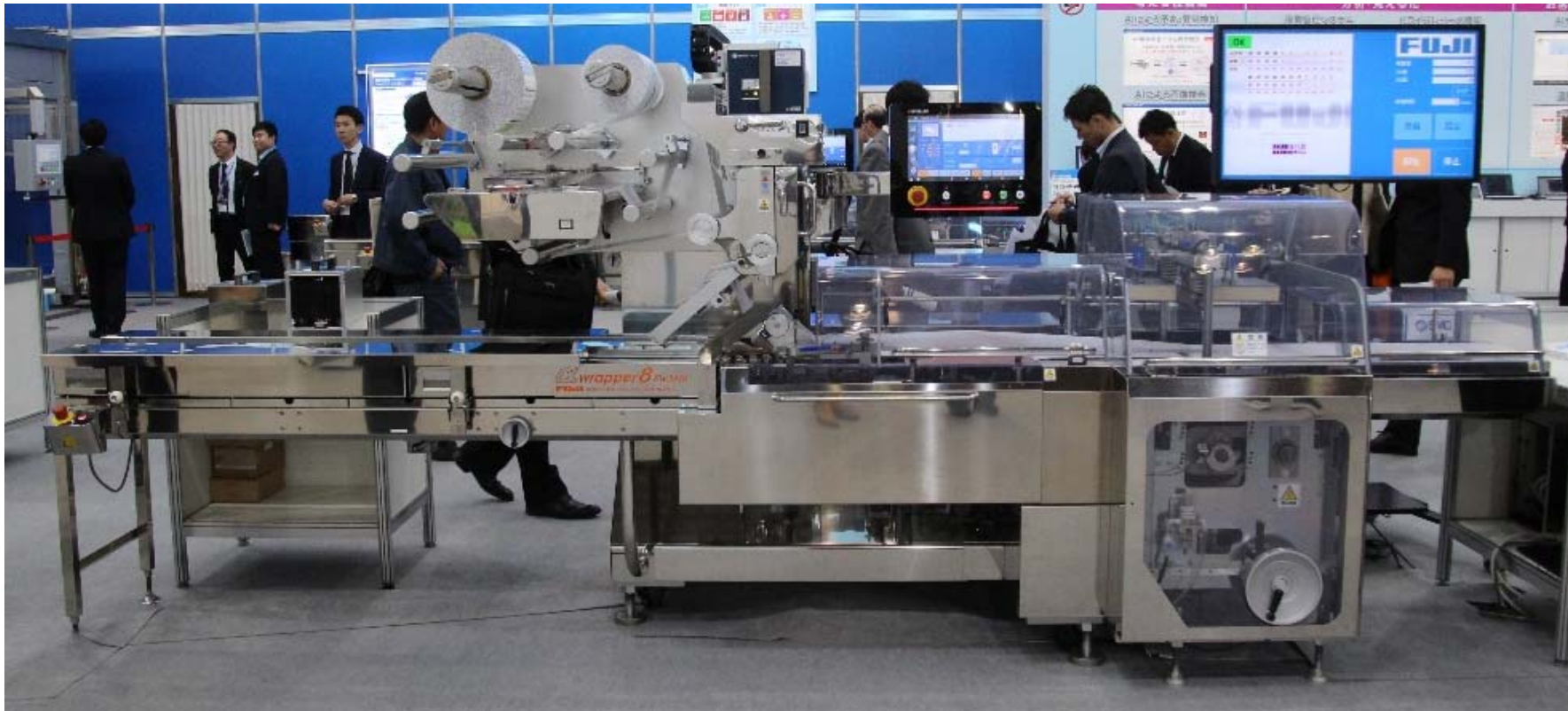
A FUJI MACHINERY high speed horizontal pillow packaging machine displayed at JAPAN PACK 2019 (the Vx 3-A is in the upper center)
