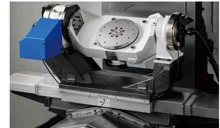
Equipped with a large tilting rotary table for machining large parts and multiple surfaces
