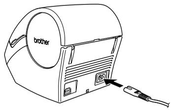
**2** Plug the AC power cord into a standard electrical outlet.
