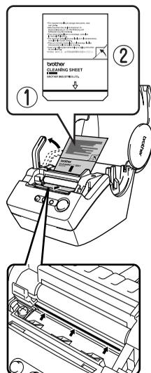
**5 After the Cleaning Sheet is inserted in the slot, peel off section (②) of the sheet.**
