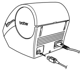
**9 Check that the QL-500/550 is turned on, and then plug the connector on the USB cable into the USB port on your personal computer.**
