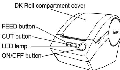
! If the DK Roll compartment cover is left open, dust will collect on the print head. Always close the cover.
