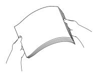
2 Unfold the paper support, and press and slide the paper guide to fit the paper width.
