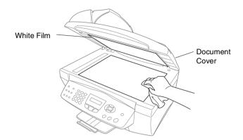
Open the document cover. Clean the white film and the glass strip under the film with isopropyl alcohol on a lint-free cloth.
