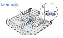
6 Squeeze the right width guide and slide it to fit the paper size.
