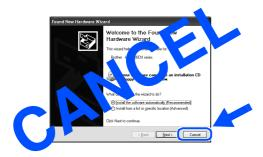
Make sure the USB interface cable is NOT connected to the printer, and then begin installing the driver. If you have already connected the cable, remove it.
