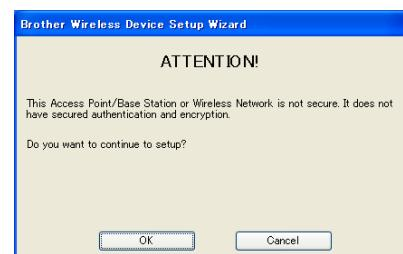
**10** When configuring your Brother Wireless device, you must ensure that it is configured to match the Authentication and Encryption settings of our existing wireless network. If your network is configured for Authentication and Encryption, choose the **Authentication Method** and **Encryption Mode** from the pull downs in each setting box. Then enter the **Network Key** and click **Next**.
