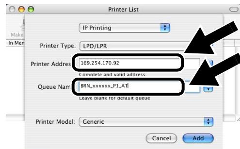
You can find the TCP/IP address by printing out the Network Configuration Page. See Other Information in this Quick Setup Guide for information how to print the Network Configuration Page.
