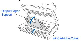
4 Remove the yellow plastic protective cartridges.
