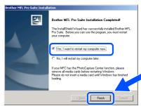
After the computer restarts, click **Yes** to have the Control Center loaded each time Windows is started. The Control Center will appear as an icon in the task tray. If you click **No** the **Scan to** keys on the MFC will be disabled.
