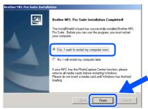
24 After the computer restarts, click Yes to have the Control Center loaded each time Windows<sup>®</sup> is started. The Control Center will appear as an icon in the task tray. If you click No the Scan to keys on the MFC will be disabled.
