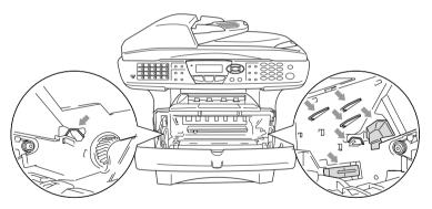
**3** Hold down the lock lever on the right and pull the toner cartridge out of the drum unit. (See *Replacing the toner cartridge* on page 22-27.)
