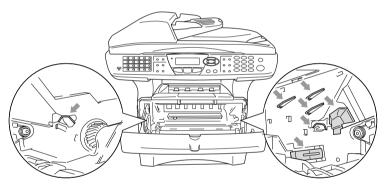
**2** Hold down the lock lever on the right and pull the toner cartridge out of the drum unit.
