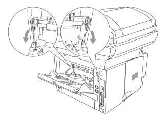
**5** Put the envelopes in the MP tray so that they touch the back of the tray. Do not put more than 3 envelopes in the MP tray at any one time, or it may cause a jam.
