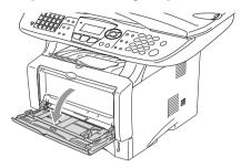
**2** Pull out and unfold the MP tray support flap.
