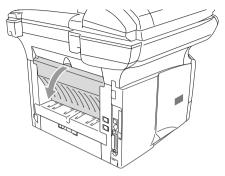
**3** Open the manual feed tray. Slide the paper guides to fit the envelope size.
