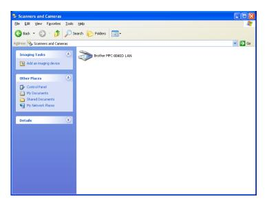
Right-click Scanner Device icon and select properties to view the Network Scanner Properties dialog box.
