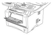
**2** Using both hands put paper in the manual feed tray until the front edge of the paper touches the paper feed roller. Hold the paper in this position until the MFC automatically feeds the paper in for a short distance, and then let go of the paper.
