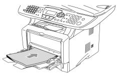
Make sure that the paper is straight and in the proper position on the MP tray. If it is not, the paper may not be fed properly, resulting in a skewed printout or a paper jam.
