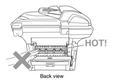
**6** Open the jam clear cover (fuser cover). Pull the jammed paper out of the fuser unit.
