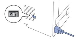
2 Plug the power cord into an AC outlet. Turn the power switch on.
