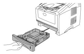
**2** While pressing the paper guide release lever, slide the adjusters to fit the paper size.
