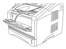
**2** Using both hands put paper in the manual feed tray until the front edge of the paper touches the paper feed roller. Hold the paper in this position until the MFC automatically feeds the paper in for a short distance, and then let go off the paper.
