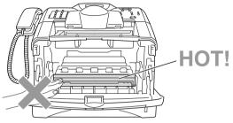
**1** Open the front cover and pull out the drum unit.
