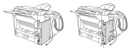
3 Loosen the two screws, and then remove the metal cover plate.
