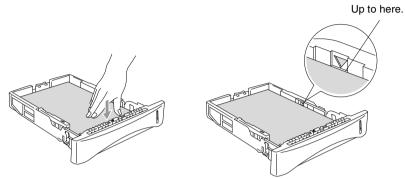
**5** Put the paper tray firmly back in the MFC and unfold the support flap before you use the MFC.
