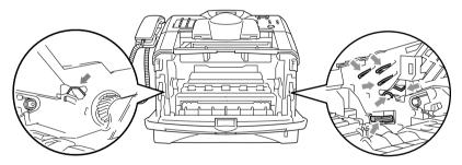
**3** Hold down the lock lever on the right and pull the toner cartridge out of the drum unit. (See *Replacing the toner cartridge* on page 12-25.)
