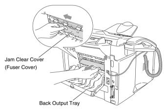
7 Close the jam clear cover (fuser cover). Close the back output tray.
