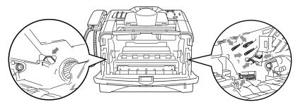
**2** Hold down the lock lever on the right and pull the toner cartridge out of the drum unit.
