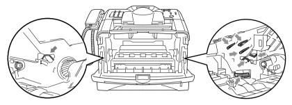
**5** Open the back output tray. Pull the jammed paper out of the fuser unit. If the paper jam can be cleared, go to Step 7.
