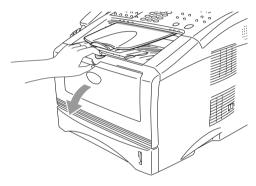
4 Pull out the drum unit and toner cartridge assembly. Pull the jammed paper up and out of the MFC. If you cannot remove the drum unit and toner cartridge assembly easily at this time, do not use extra force. Instead, pull the edge of the jammed paper out of the paper tray. If the jammed paper can not be pulled out easily, turn the jam dial towards you so that you gently pull the paper out.
