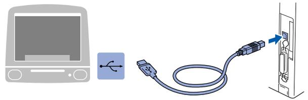
**Do not connect the MFC to a USB port on a keyboard or a non powered USB hub.**
