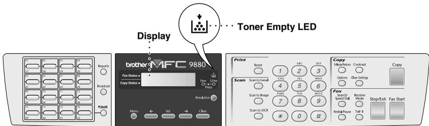
The Toner Empty LED light stays on and the display shows **TONER EMPTY** to indicate that the toner is empty. Once this indication appears, the machine will not resume printing until you have installed a new toner cartridge.
