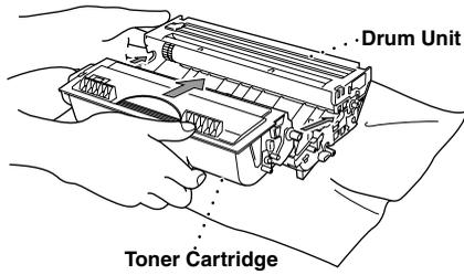
**7** Clean the primary corona wire inside the drum unit by gently sliding the blue tab from right to left several times. Return the blue tab to the home position before reinstalling the drum unit assembly.
