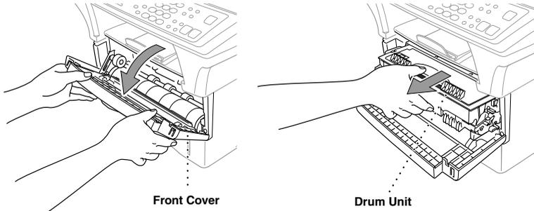
Place the drum unit on a drop cloth or large piece of disposable paper to avoid spilling and scattering the toner.
