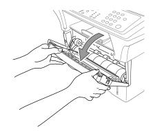
**D.** Insert the drum unit assembly into the machine.
