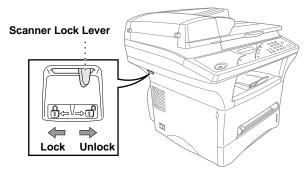
If CHECK SCAN LOCK appears on the LCD, check the lever is fully in the unlock position and press Stop.
