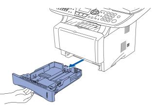
2 While pressing the paper guide release lever, slide the adjusters to fit the paper size. Check that the guides are firmly in the slots on the tray.
