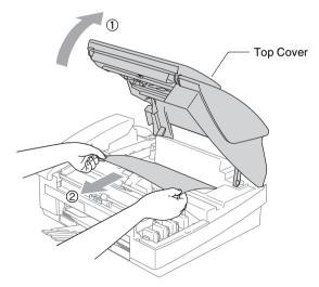
If the paper is jammed underneath the print head, disconnect the machine from the power source so you can move the print head to take out the paper.
