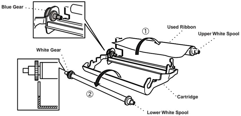
**4** Slide the white elastic off the new refill rolls and set them down with the full roll in the lower position. (The ribbon's shiny side is facing *down*.)
