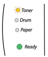
The **Toner** LED alternates turning on for 2 seconds and off for 3 seconds.
