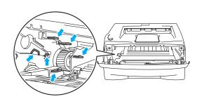
4 Push down the blue lock lever and take the toner cartridge out of the drum unit.
