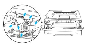
3 Clean the primary corona wire inside the drum unit by gently sliding the blue tab from right to left and left to right several times. Return the tab to the home position (▲) before you put the drum unit back in the printer. If you do not, printed pages may have a vertical stripe.
