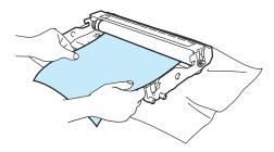
2 Turn the drum unit gear by hand while looking at the surface of the OPC drum.
