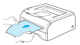
3 Remove the printed even-numbered pages from the output tray and put them back into the manual feed slot in the same order one by one. Place the paper with the side that is going to be printed on (the blank side) face up. Follow the instructions on the computer screen.
