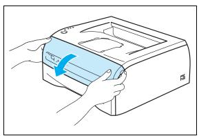
3 Pull out the drum unit and toner cartridge assembly.
