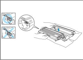
Put the drum unit and toner cartridge assembly back in the printer.
