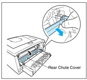
7 Pull the jammed paper out of the fuser unit. If the jammed paper cannot be pulled out easily, push down the tab with one hand as you gently pull the paper out with other.
