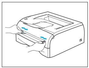
5 Using both hands, put one piece of paper or one envelope in the manual feed slot until the front edge of the paper or envelope touches the paper feed roller. When you feel the machine pull in the paper, let go.
