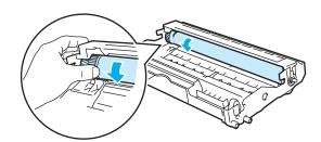
3 When you have located the mark on the drum that matches the print sample, wipe the surface of the OPC drum with a cotton swab until the dust or paper powder on the surface comes off.
