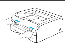
5 Using both hands, put one piece of paper or one envelope in the manual feed slot until the front edge of the paper or envelope touches the paper feed roller. When you feel the machine pull in the paper, let go.
