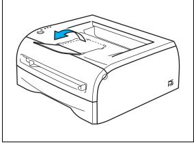
4) Using both hands, slide the manual feed slot paper guides to the width of the paper that you are going to use.
