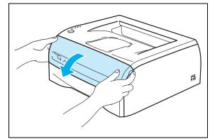
Pull out the drum unit and toner cartridge assembly.
