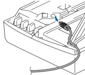
3. Carefully guide the USB cable into the trench as shown below, following the trench round and toward the back of the machine.
