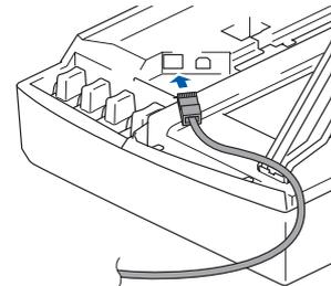
3. Carefully guide the network cable into the trench as shown below, following the trench round and toward the back of the machine.
