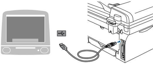
**DO NOT** connect the machine to a USB port on a keyboard or a non-powered USB hub.
