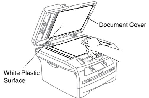
In the ADF unit, clean the white plastic bar and the scanner glass strip under it with isopropyl alcohol on a lint-free cloth.
