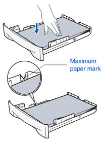
5 Put the paper tray firmly back into the machine and unfold the output paper tray support flap before you use the machine.
