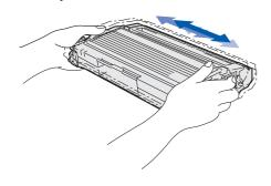
4 Put the drum unit assembly into the machine.
