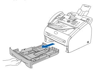
While pressing the paper guide release lever, slide the adjusters to fit the paper size. Check that the guides are firmly in the slots.
