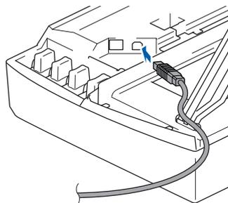
**12** Carefully route the USB cable through the trench and out the back of the machine as shown below.
