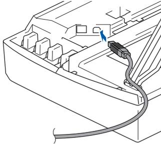
**10** Carefully route the USB cable through the trench and out the back of the machine as shown below.
