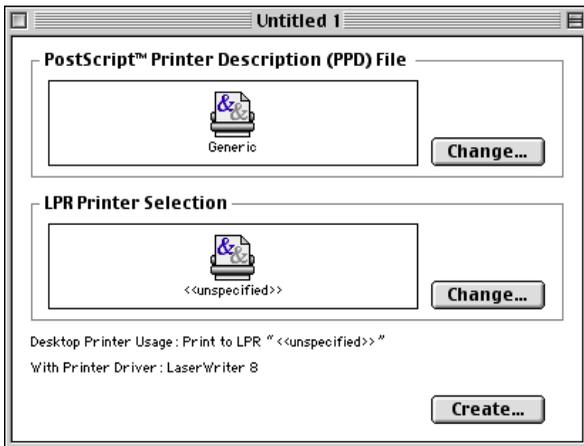
**Figure 4 Selecting the PPD and LPR Configuration**
