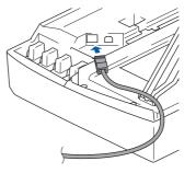
**10** Carefully guide the network cable to the trench as shown below, following the trench around and toward the back of the machine. Then, connect the cable to your network.
