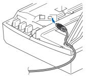
Carefully guide the USB cable into the trench as shown below, following the trench around and toward the back of the machine.
