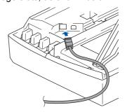
Carefully guide the network cable into the trench as shown below, following the trench around and toward the back of the machine. Then, connect the cable to your network.
