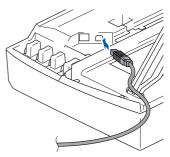
**12** Carefully guide the USB cable into the trench as shown below, following the trench around and toward the back of the machine.
