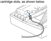
Carefully guide the network cable into the trench as shown below, following the trench around and toward the back of the machine. Then, connect the cable to your network.
