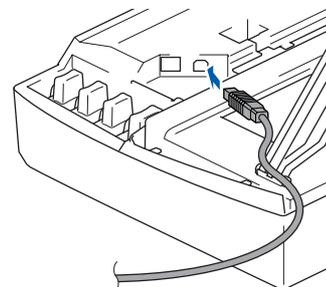
**10** Carefully guide the USB cable into the trench as shown below, following the trench around and toward the back of the machine.
