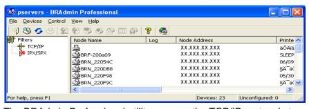
The BRAdmin Professional utility can use the TCP/IP protocols to communicate with the Brother Print/Scan server.
