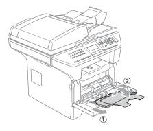
3 Insert the media into the MP tray with the top edge first and the printing side face up.
