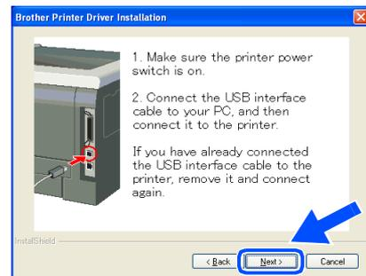
Installing the driver and connecting the printer to your PC
